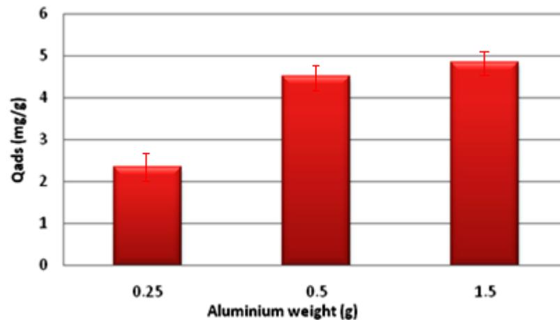
Figure 7. Effect of aluminum mass on adsorption long-wave.
