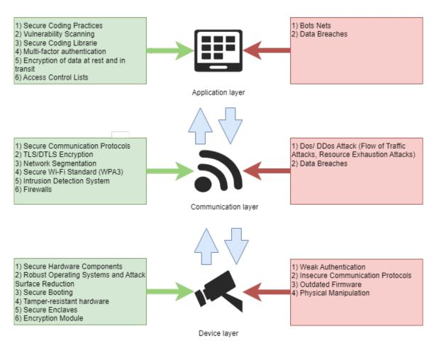
Figure 6. Common threats in the IoT with corresponding defenses.
