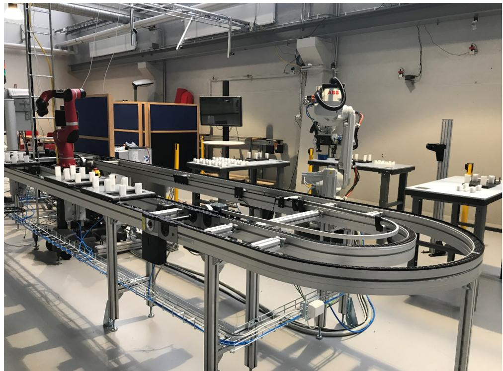
**Figure 8.** Physical setup of HRC assembly workstations.
