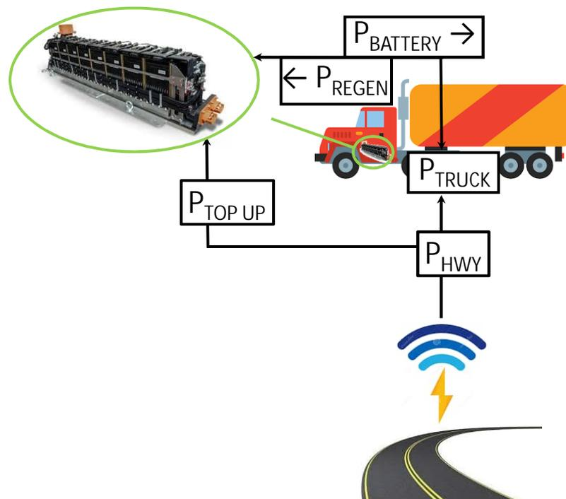
**Figure 4.** Power flow configuration for simulation EHT. The inset in the green oval shows the truck battery pack.
