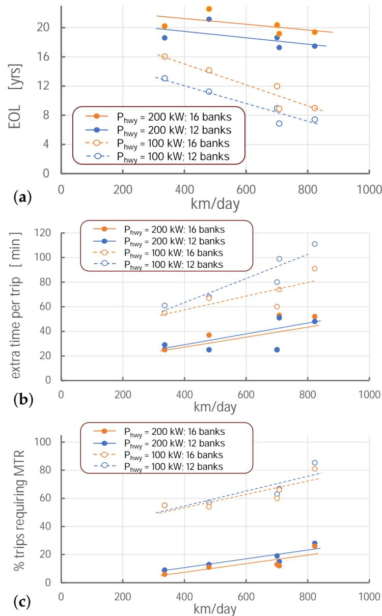
**Figure 12.** Lifetime characteristics of the five EHTs operating on low power e-Hwys where mid-trip recharging operations were permitted. Plots versus daily average driving distance: (a) EOL given in years, (b)  $t_{extra}$  in minutes per day, and (c) percentage of trips requiring mid-trip recharge.
