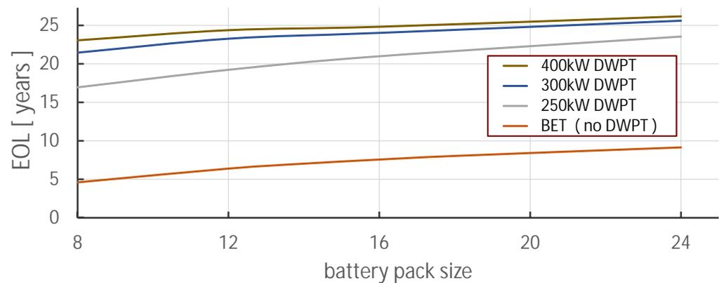
**Figure 11.** EOL vs battery pack size (in banks) for EHTs at 250, 300 and 400 kW  $P_{\text{hwy}}$  levels, average value for all five trucks. Also shown is an EOL curve for a BET with the same range of battery pack sizes.
