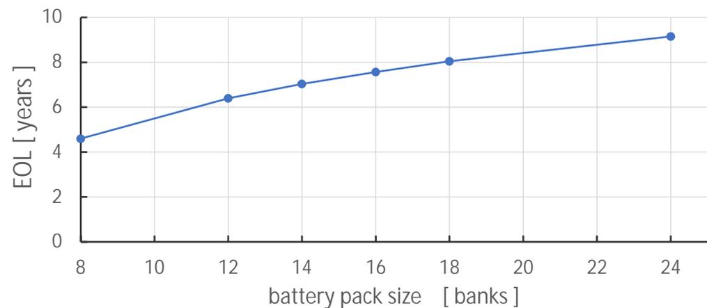
**Figure 7.** Battery pack EOL versus pack size using on-road driving profiles for BETs with megawatt charging.
