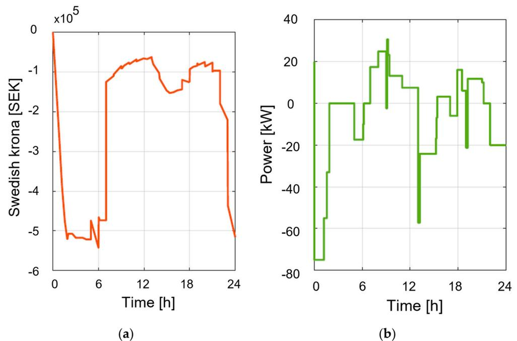
**Figure 7.** The price (SEK) in (a) and power (kW) to or from the grid in (b) to cover the charging and discharging of the 10 EVs over one day (hour).
