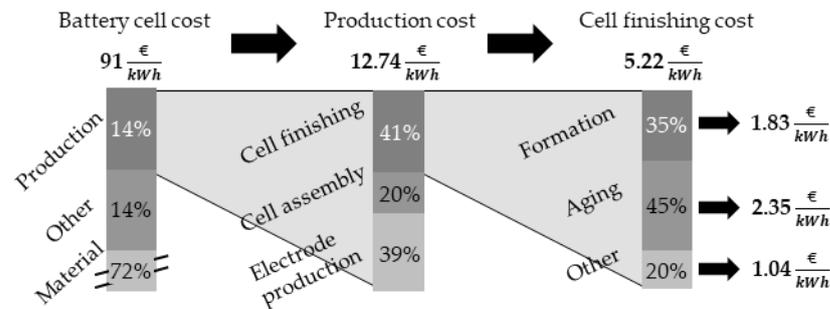
**Figure 1.** Distribution of OPEX within battery production.
