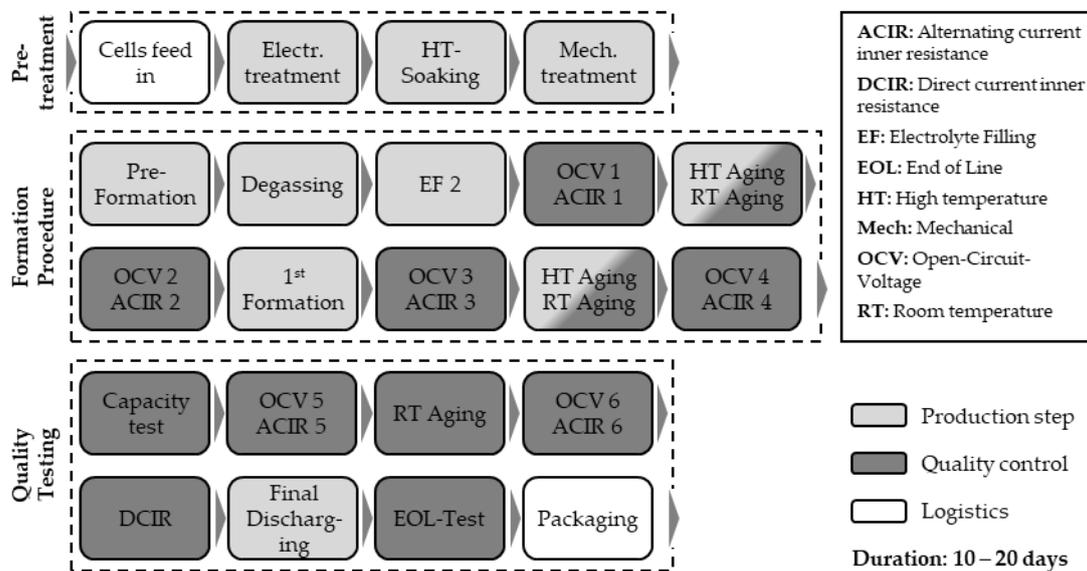
Figure 2. Example cell finishing process route [7].
