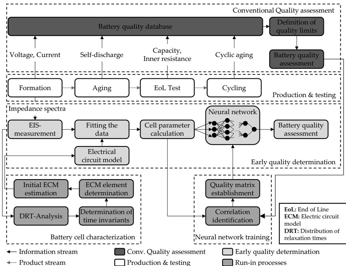
**Figure 5.** Implementation concept for an EIS-based early quality determination.
