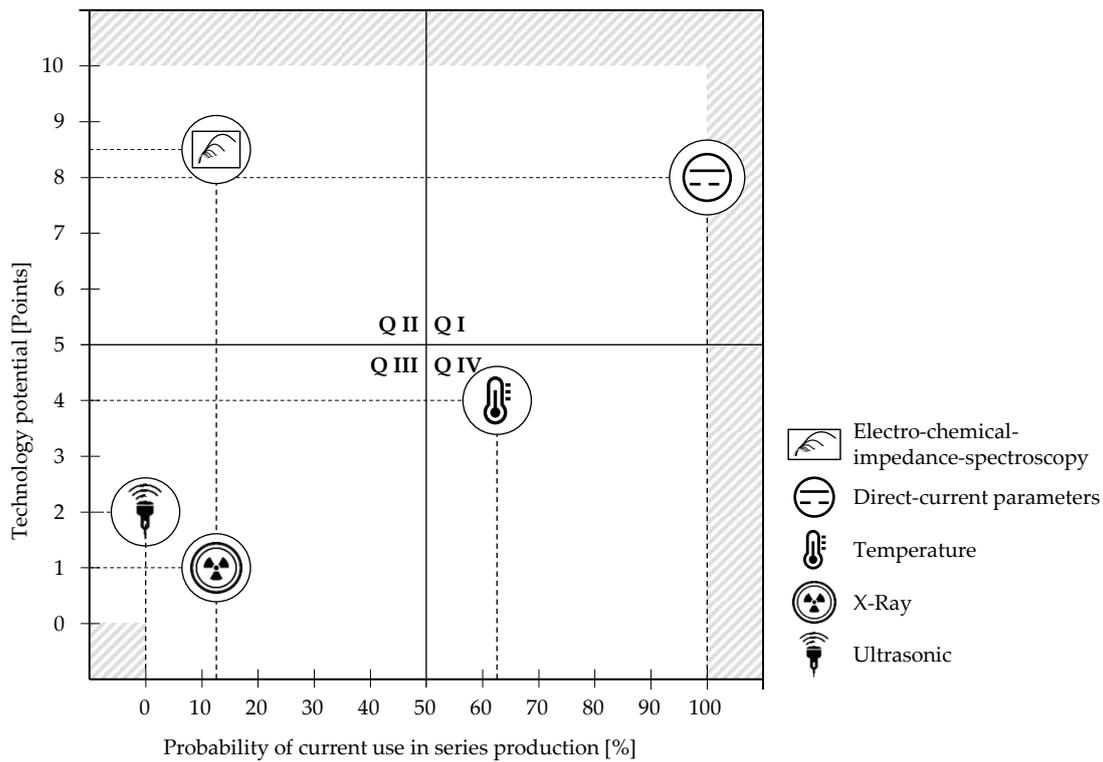
**Figure 4.** Technology potential for early quality determination in comparison to the current implementation in series productions.
