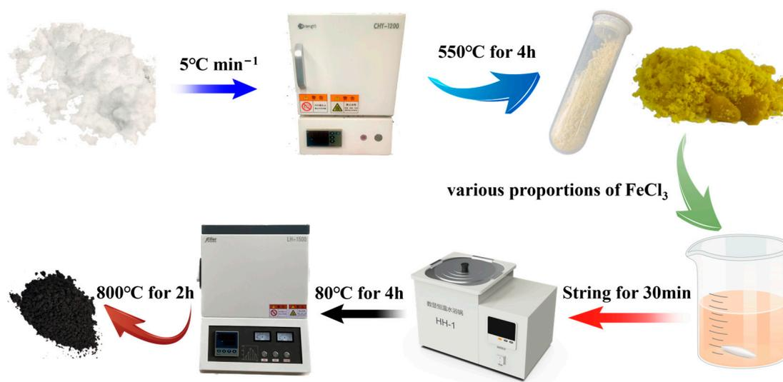
Figure 1. The preparation diagram of the Fe-NC catalyst.
