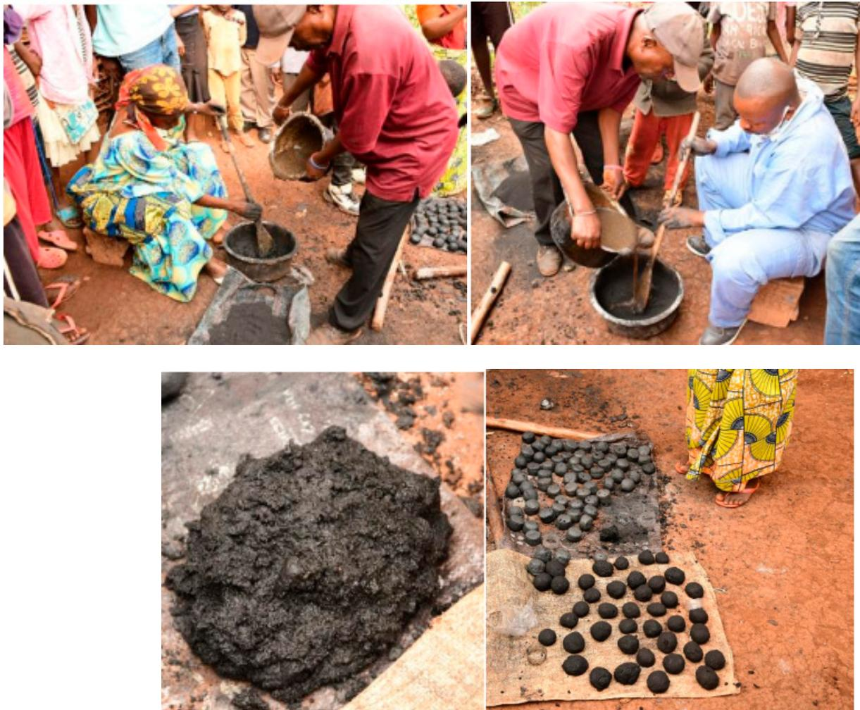
**Figure 5.** Steps in making briquettes by smallholder farmers supported by a local non-governmental organization, DIOBASS, in eastern DRC.
