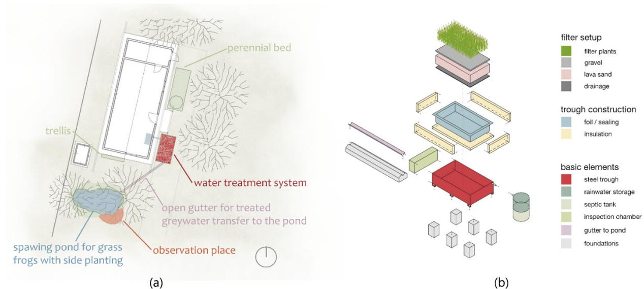
**Figure 9.** Preliminary design proposal of the students. (a) The single components were defined and brought into a spatial context. (b) The students’ axonometry shows the design of the filtration bed. The structure is based on other small greywater treatment plants (examples for comparable structures: [37,41,45]).
