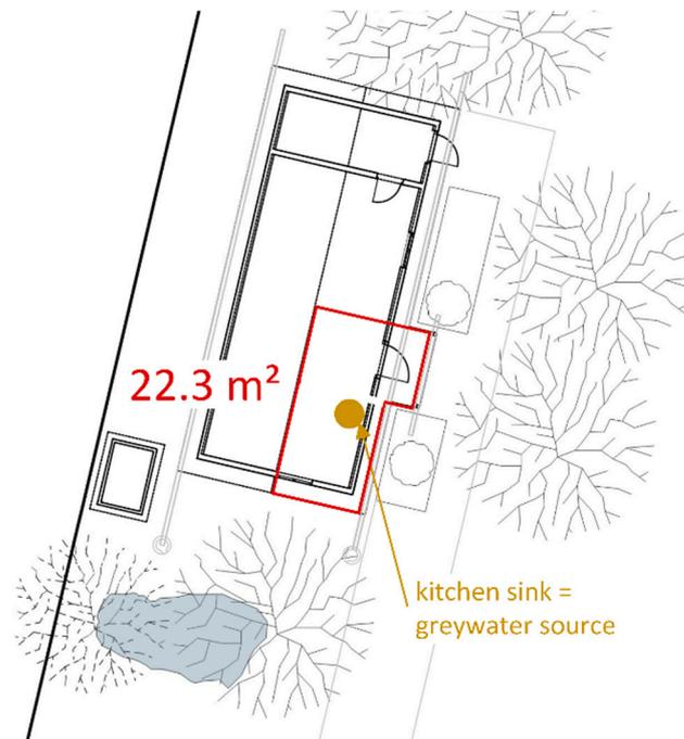
**Figure 5.** The roof area of 22.3 m<sup>2</sup> close to the greywater source was considered for rainwater harvesting. The rainwater gutters would have to be connected to the system individually.
