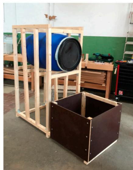
**Figure 10.** Documentation of the development of technical components for the BGA project. (a) Considerations for septic tank design and filter loading. These students' sketches do not show the final design, but an intermediate step in the planning. (b) Based on CAD drawings and 3D models, the assembly of the components was prepared. (c) The timber framework is pre-fabricated in the workshop.
