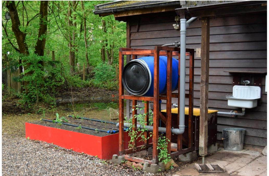
**Figure 14.** Built result of the BGA project 10 months after completion. The operation ran without any disruptions. In winter, the septic tank was bypassed. In the meantime, summer operation was resumed. The plants on the constructed wetland all survived the winter well and will grow even bigger in the next few years.
