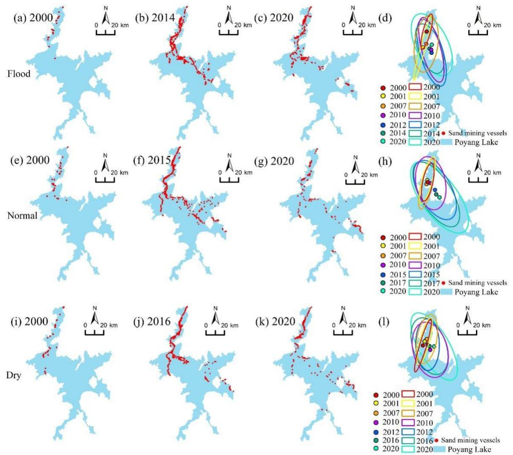
**Figure 2.** (a–c) Distribution of sand mining vessels during the flood season; (d) The standard deviation ellipse and mean center in flood season; (e–g) Distribution of sand mining vessels during the normal season; (h) The standard deviation ellipse and mean center in normal season; (i–k) Distribution of sand mining vessels during the dry season; (l) The standard deviation ellipse and mean center in the dry season.
