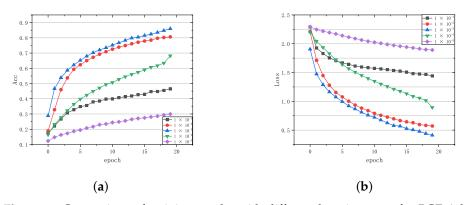
**Figure 1.** Comparison of training results with different learning rates for BGE-Adam settings. (a) Comparison of accuracy values for different learning rates; (b) Comparison of loss values for different learning rates.
