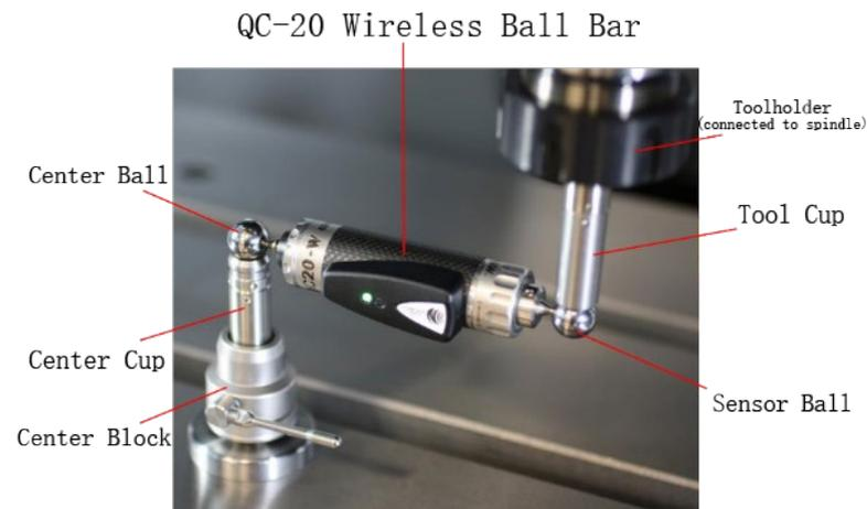
**Figure 18.** QC20-W double ballbar system.
