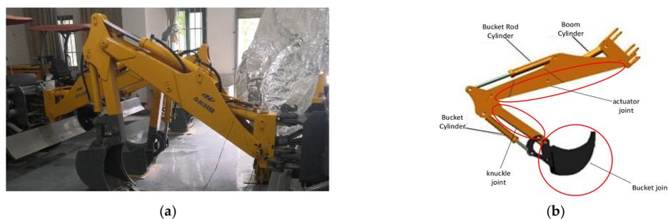
**Figure 1.** Excavator research model. (a) The prototype model of the excavator. (b) The working device of a virtual prototype model.
