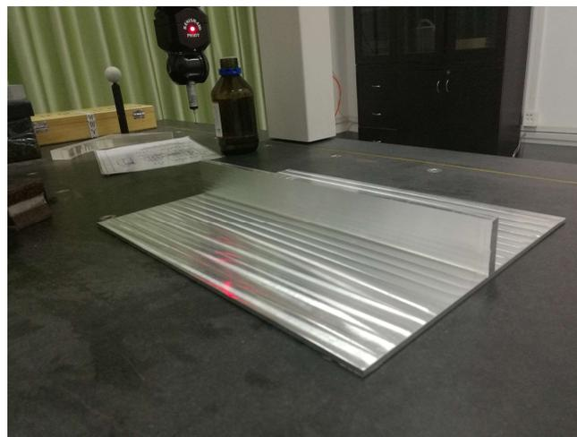
Figure 15. Measurement of Machining Deformation of T-shaped Component.
