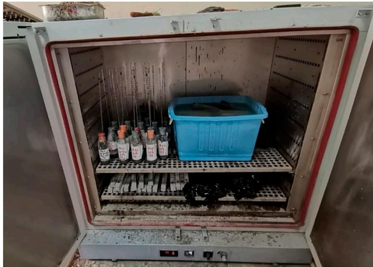
**Figure 4.** Samples for length change and mechanical property testing, placed in an oven at a constant temperature of 45 °C.
