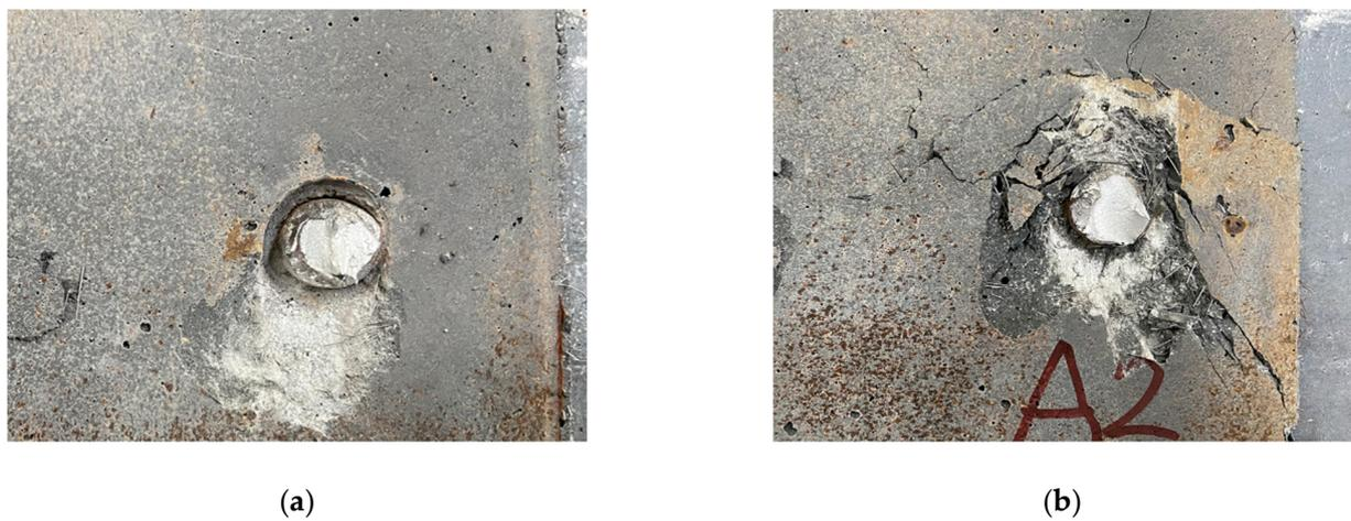
Figure 6. Failure modes of UHPC. (a) Mode A. (b) Mode B.
