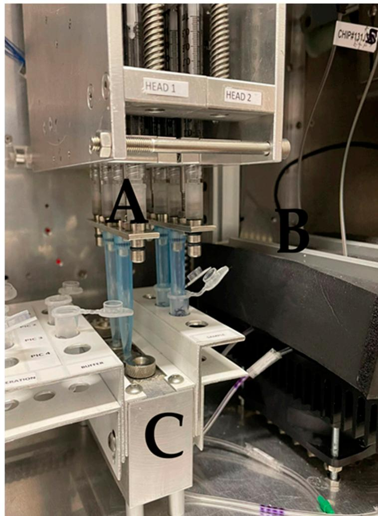
**Figure 1.** The novel POC device. (A) Syringe system for buffer/sample delivery. (B) Insulating material that covers the PICs and in combination with the Peltier element maintains a steady temperature of 25 °C during analysis. (C) Sample and buffer holder. The circular metallic inlets of the microfluidic system are shown.
