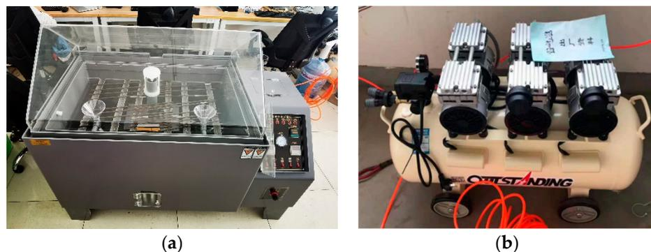
**Figure 1.** Salt spray test equipment. (a) Salt spray chamber, (b) Air compressor.
