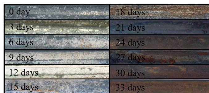
**Figure 4.** Macroscopic surface of corroded steel wire.
