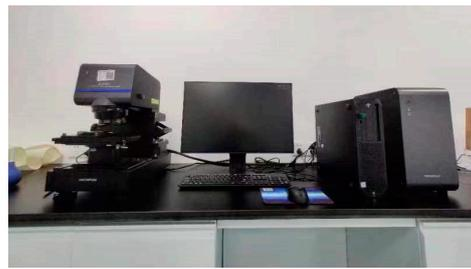
Figure 9. Confocal Laser Scanning Microscope.
