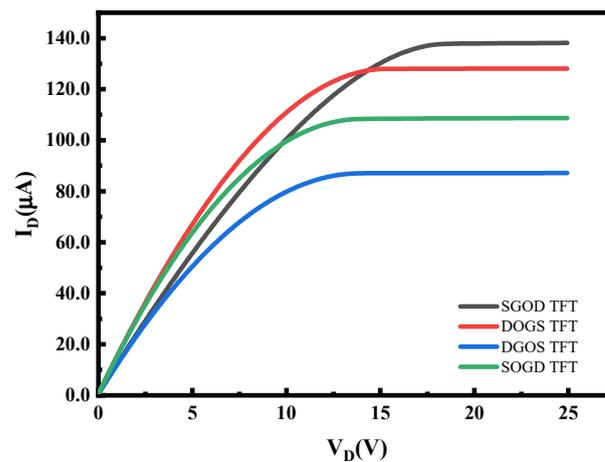
**Figure 4.** The theoretical output characteristics of different offset Corbino TFTs with the same  $L_{offset}$  of 10 μm and the same  $L_{channel}$  of 175 μm when  $V_G$  is 15 V.
