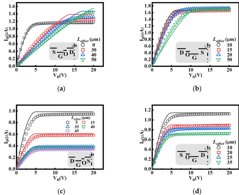
Figure 8. The experimental output characteristics of offset Corbino TFT when  $V_G$  is 4 V: (a) SGOD TFT. (b) DOGS TFT. (c) DGOS TFT. (d) SOGD TFT. Insets of (a–d) are the corresponding schematic of offset Corbino TFT. The dots are experimental data, and the curves are the fitting results using the derived Equations.
