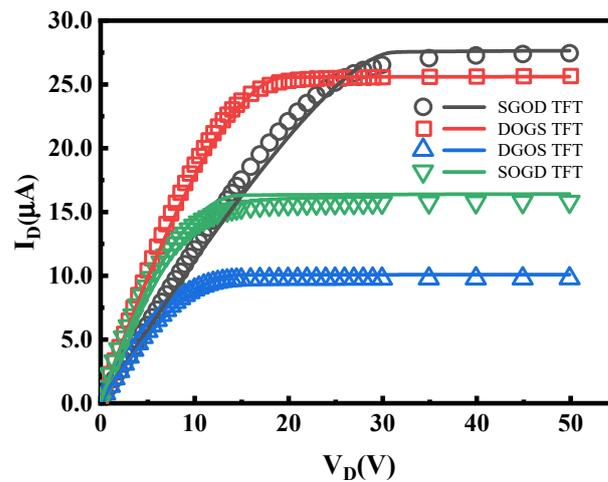
**Figure 6.** The simulation output characteristics of different offset Corbino TFTs with the same  $L_{offset}$  of  $10\ \mu\text{m}$  and the same  $L_{channel}$  of  $175\ \mu\text{m}$  when  $V_G$  is  $15\ \text{V}$ . The TCAD simulated data are drawn in dots, and fitting results by using the derived Equations are drawn in curves.
