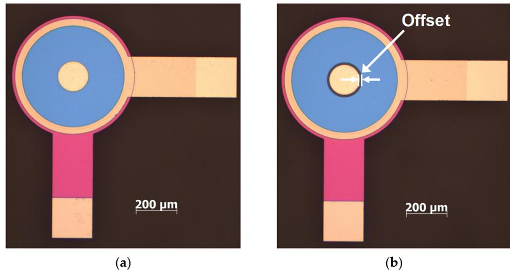
Figure 7. Optical images of fabricated a-IGZO Corbino TFTs: (a) without offset; and (b) with an offset of 10  $\mu\text{m}$ .
