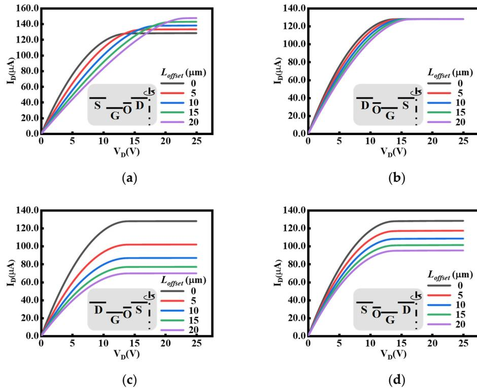
**Figure 3.** The theoretical output characteristics of offset Corbino TFT when  $V_G$  is 15 V: (a) SGOD TFT. (b) DOGS TFT. (c) DGOS TFT. (d) SOGD TFT. Insets of (a–d) are the corresponding schematic of offset Corbino TFT.
