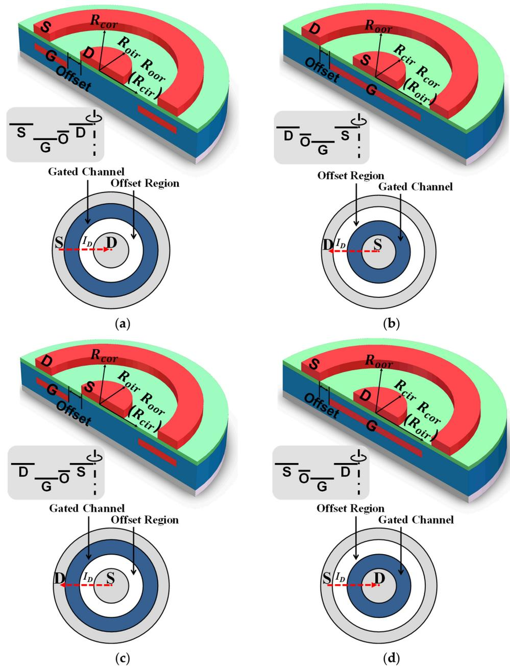
**Figure 1.** The three-dimensional cross-sectional structures and top views of offset Corbino TFTs. (a) SGOD TFT. (b) DOGS TFT. (c) DGOS TFT. (d) SOGD TFT. Insets of (a–d) are the corresponding schematic of offset Corbino TFTs.
