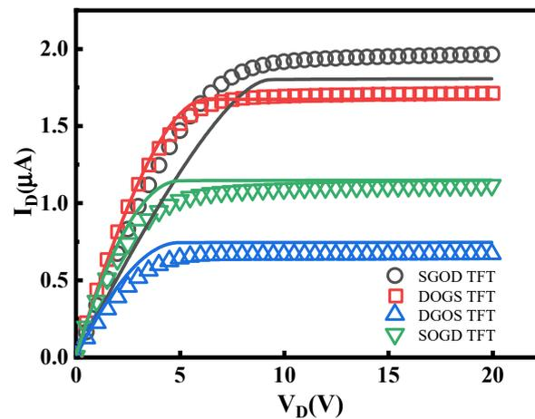
**Figure 9.** The experimental output characteristics of different offset Corbino TFTs with the same  $L_{offset}$  of 10  $\mu\text{m}$  and the same  $L_{channel}$  of 175  $\mu\text{m}$  when  $V_G$  is 4 V. The dots are experimental data, and the curves are the fitting results by using the derived Equations.
