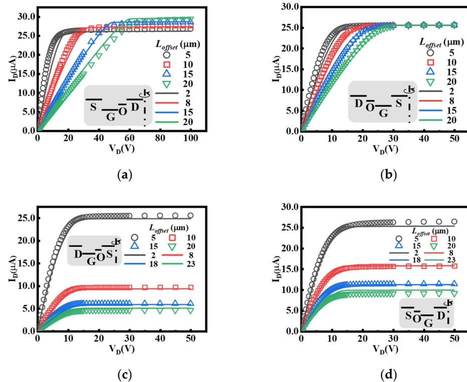
**Figure 5.** The simulation output characteristics of offset Corbino TFT when  $V_G$  is 15 V: (a) SGOD TFT. (b) DOGS TFT. (c) DGOS TFT. (d) SOGD TFT. Insets of (a–d) are the corresponding schematic of offset Corbino TFT. The TCAD simulated data are drawn in dots, and relevant results using the derived Equations are drawn in curves.
