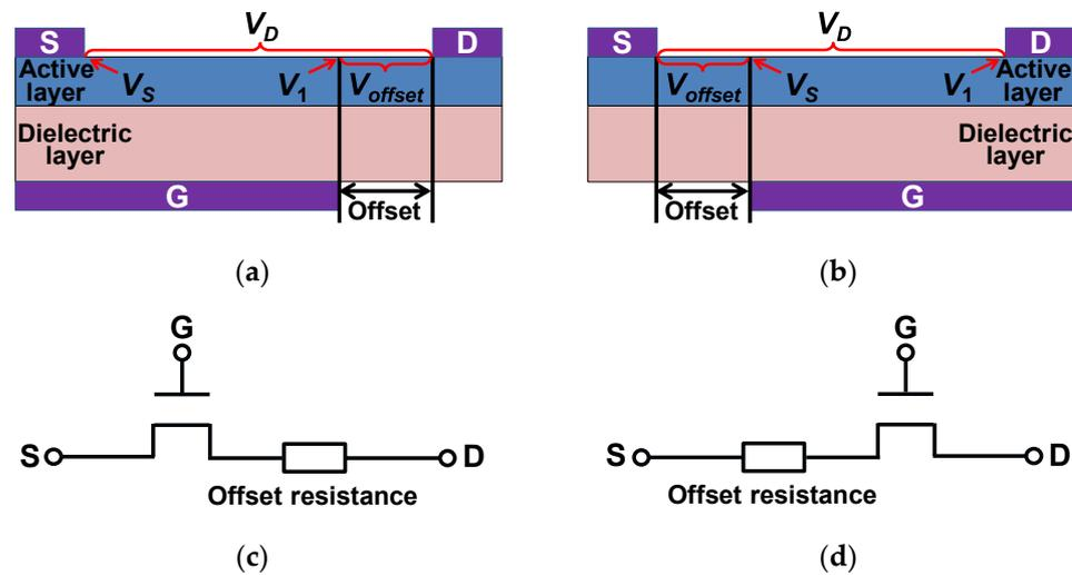
**Figure 2.** The cross-section image of (a) Drain-Offset Corbino TFT, and (b) Source-Offset Corbino TFT. The schematic diagram of the equivalent circuit of (c) Drain-Offset Corbino TFT, and (d) Source-Offset Corbino TFT.
