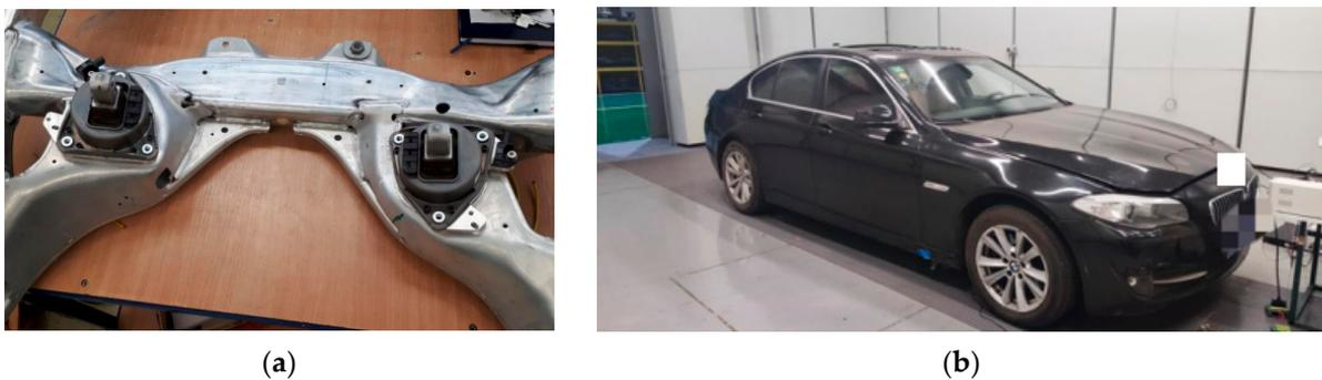
**Figure 9.** Rapid control prototype test platform. (a) Subframe fitted with electro-hydraulic composite engine mounts; (b) modified test vehicle.
