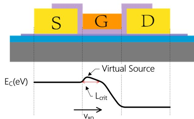
**Figure 1.** Schematic diagram of the energy band structure of a CNTFET.
