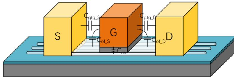
Figure 2. Capacitance in CNTFETs.
