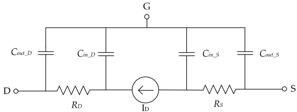
Figure 4. Equivalent circuit of the VSEX model.
