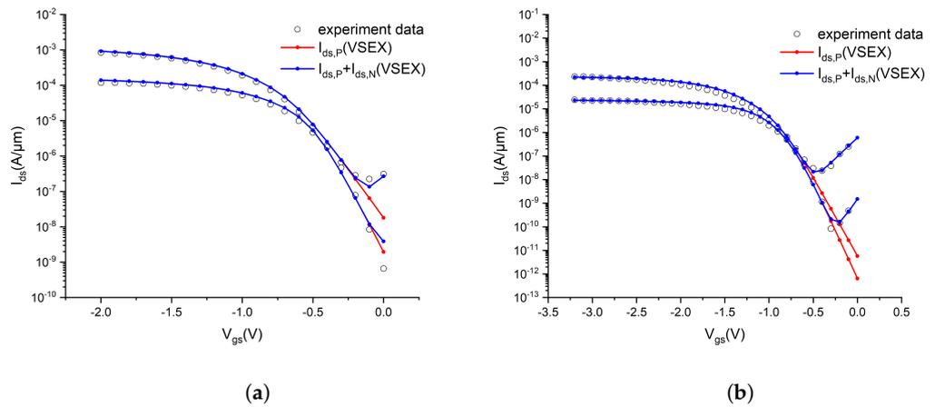
Figure 7. P-type CNTFET transfer characteristic. (a)  $L_C = 200$  nm; (b)  $L_C = 2$   $\mu$ m.
