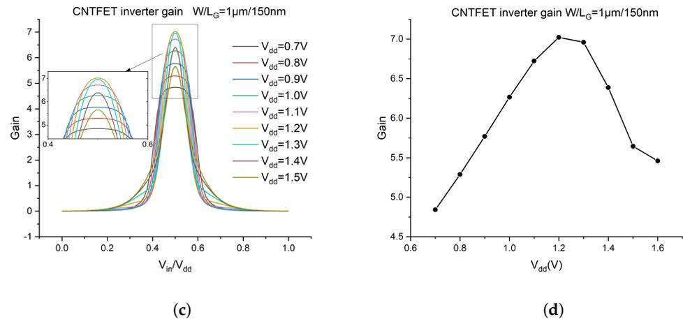
**Figure 8.** Inverter based on CNTFETs with  $L_G = 150$  nm. (a) The structure of inverter; (b) inverter output curves; (c) gain of inverter; (d) gain versus  $V_{dd}$ .
