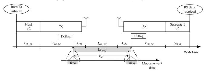
Figure 4. WSN time delay characterization for WSN communication channel.
