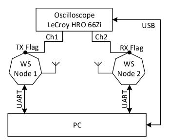
Figure 6. Experimental setup for time delay distribution characterization.
