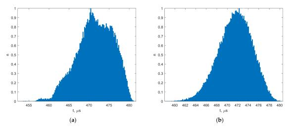
**Figure 12.** SX1276 FSK histogram modeled for data packet re-transfer: (**a**) through 2 nodes; (**b**) through 4 nodes.
