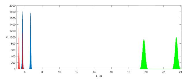
Figure 7. NRF24L01 delay histograms: green—250 kbps; blue—1000 kbps; red—2000 kbps.
