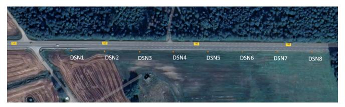
Figure 3. Animal detection IoT network with the implemented placement of the DSN nodes.
