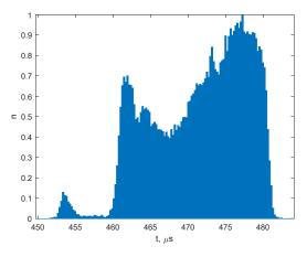
Figure 11. SX1276 FSK histogram measured using point-to-point setup.
