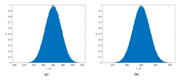
**Figure 14.** SX1231 OOK histogram modeled for data packet re-transfer: (a) through 2 nodes; (b) through 4 nodes.
