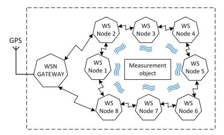
Figure 1. WSN structure with receiver–receiver synchronization.
