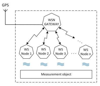
Figure 2. WSN structure with sender–receiver synchronization.
