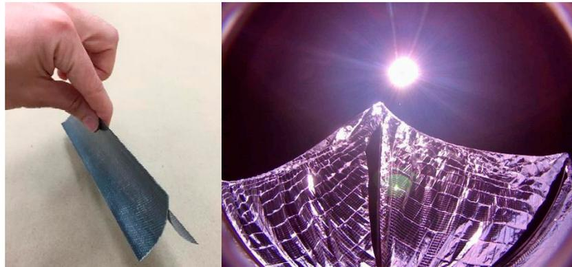
Figure 4. Membrane structure prototype with TRAC tape-spring booms launched by NASA [16].
