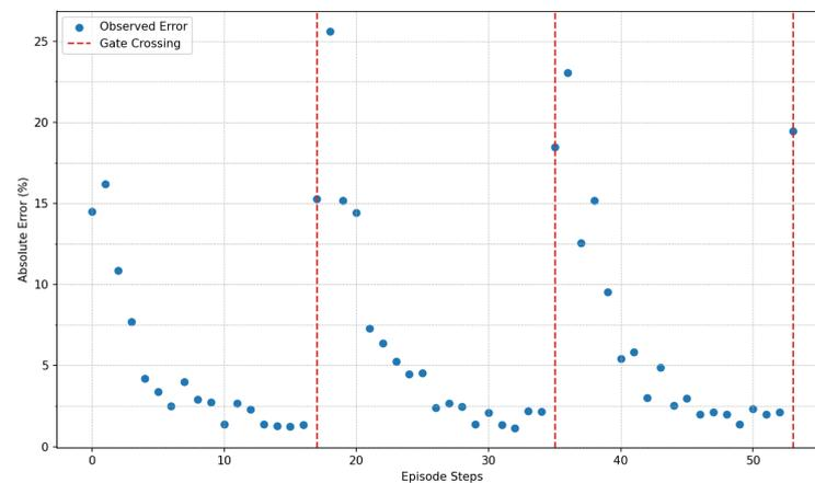
**Figure 4.** Absolute observed error between the predicted and simulated gate's center position at the crossing time for a given episode is detailed. An increase in error is noted when the IMM filter transitions to target the next gate. However, this error quickly reduces to below 5 percent, indicating rapid adjustment and improved prediction accuracy post-transition.
