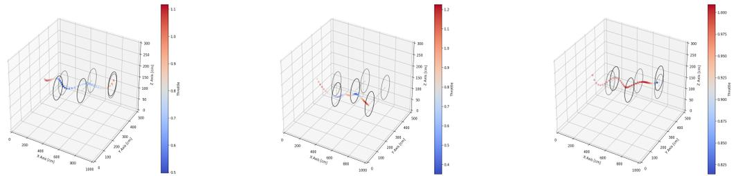
**Figure 7.** Visualization of the agent's trajectory for different training steps, showing progressively optimized and faster performance in flying through the gates with more training steps.
