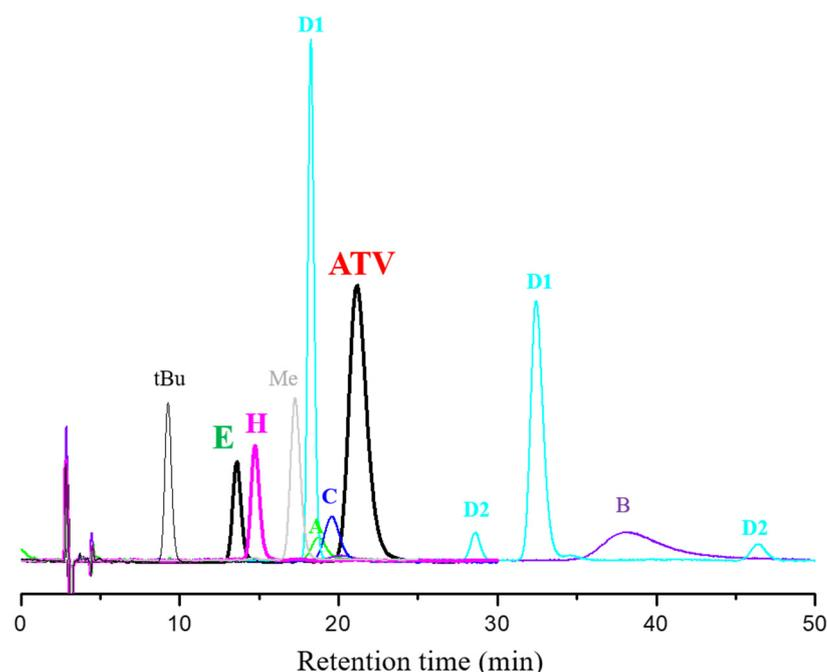
**Figure 2.** Chromatograms pertinent to the sequential HPLC analysis of the mixture IMP-E(E)/ATV and the single impurities IMP-A (A), IMP-B (B), IMP-C (C), IMP-D (D1 + D2), IMP-H (H), IMP-OMe (Me), and IMP-OtBu (tBu). Chromatographic conditions: column, Chiralpak AD-3 (250 mm  $\times$  4.6 mm, 3  $\mu$ m); mobile phase, n-hexane-ethanol-TFA 90:10:0.1 (v/v/v); flow rate, 1.0 mL min<sup>-1</sup>; temperature, 25  $^{\circ}$ C; detection, UV at 254 nm.
