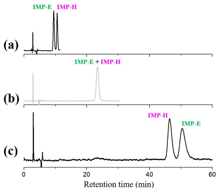
**Figure 5.** Typical HPLC chromatograms showing the inversion of the elution order of the impurities E and H. Chromatographic conditions: column, Chiralpak AD-3 (250 mm  $\times$  4.6 mm, 3  $\mu$ m); mobile phase, (a) n-hexane-ethanol-FA 89:11:0.1 (v/v/v), (b) n-hexane-ethanol-FA 93:7:0.1 (v/v/v), (c) n-hexane-ethanol-FA 95:5:0.1 (v/v/v); flow rate, 1.0 mL min<sup>-1</sup>; temperature, 35  $^{\circ}$ C; detection, UV at 254 nm.
