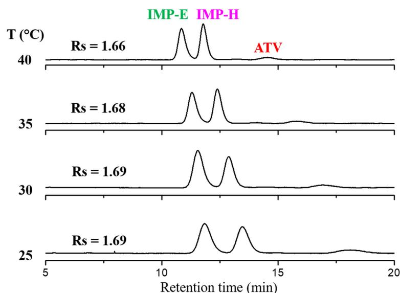
**Figure 3.** Variable temperature HPLC resolution of impurities E and H. Chromatographic conditions: column, Chiralpak AD-3 (250 mm × 4.6 mm, 3 μm); mobile phase, n-hexane-ethanol-FA 90:10:0.1 (v/v/v); flow rate, 1.0 mL min<sup>-1</sup>; temperature, 25, 30, 35, and 40 °C; detection, UV at 254 nm.
