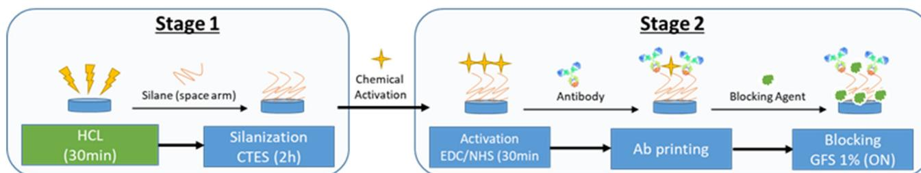
Figure 1. Graphic representation of PIC functionalization process ([46]).
