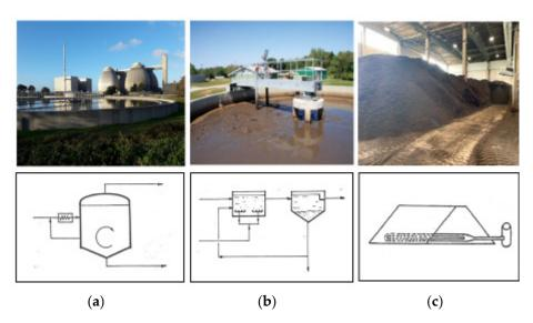
Figure 4. View of (a) anaerobic digestion, (b) aerobic stabilization, and (c) windrow composting.
