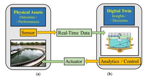
Figure 6. Mode of action of digital twins: (a) real plant, (b) virtual plant.
