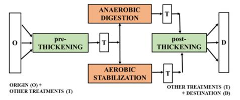
Figure 2. Technical "Hubs" in sludge processing from origin to destination.
