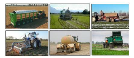
Figure 5. Examples of vehicles equipped for handling sludge/biosolids of different physical consistencies.
