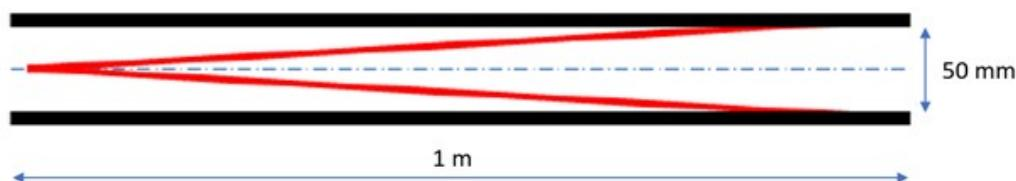
**Figure 6.** Top view of the FOM assembly, which provides a well-defined wavelength band of 2–15 Å.
