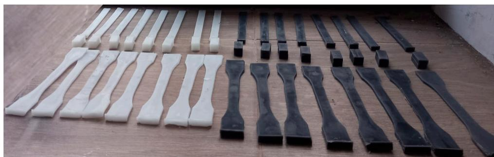
**Figure 4.** The paraffin and new propellant specimens used for the mechanical tests.
