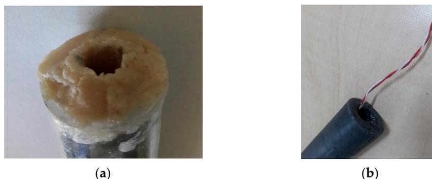
**Figure 9.** Fuel rod ignition system: (a) potassium nitrate and sugar; (b) nickeline wires for ignition.
