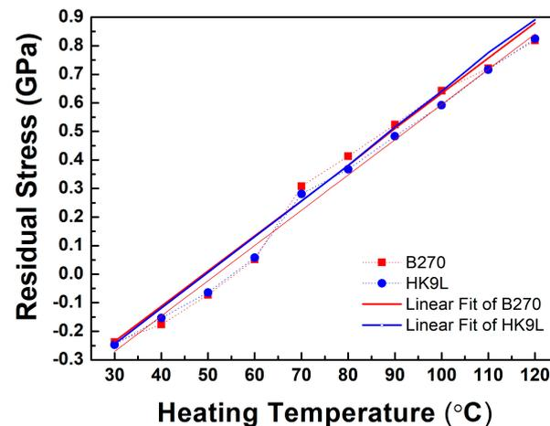
**Figure 7.** Linear fitting diagram of the residual stress vs. heating temperature for VO<sub>2</sub> film coated on B270 and H-K9L glass substrates.
