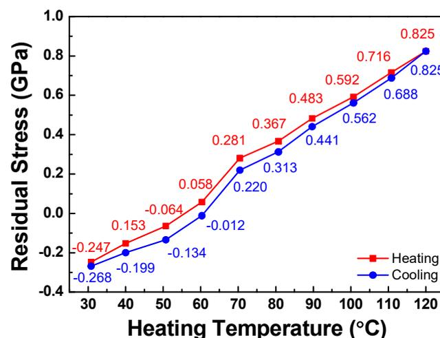
Figure 6. Residual stress vs. heating temperature for VO<sub>2</sub> film coated on H-K9L glass.
