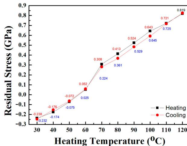
**Figure 4.** Residual stress vs. heating temperature for VO<sub>2</sub> film coated on B270 glass.
