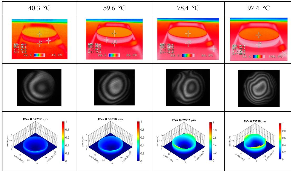
**Figure 3.** Thermal images, interference fringes, and 3D surface profile of the VO<sub>2</sub> film coated on the B270 glass substrate at different heating temperatures.
