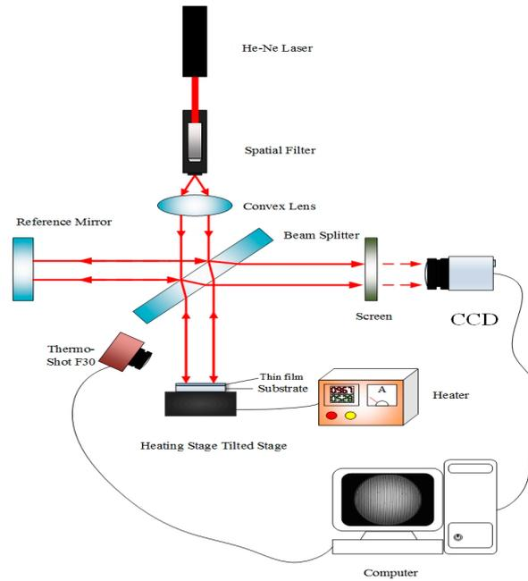
**Figure 2.** Schematic diagram of the measurement system for measuring residual stress and thermal stress.
