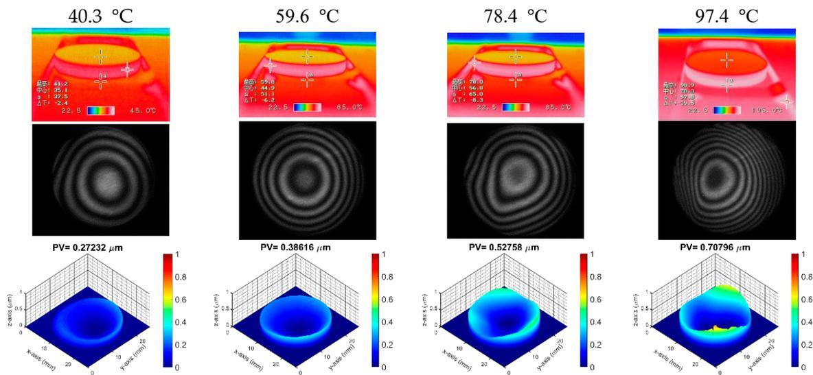
Figure 5. Thermal images, interference fringes, and 3D surface profile of the VO<sub>2</sub> film coated on the H-K9L glass substrate at different heating temperatures.
