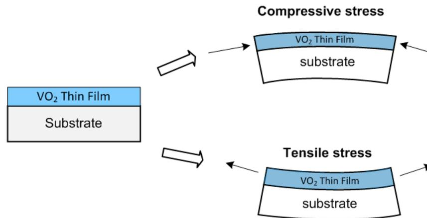
Figure 1. Schematic diagrams of the thin film/substrate system under tensile or compressive stress.
