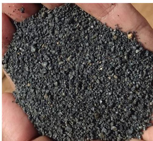
Figure 2. Waste copper slag as fine aggregate used in the study.
