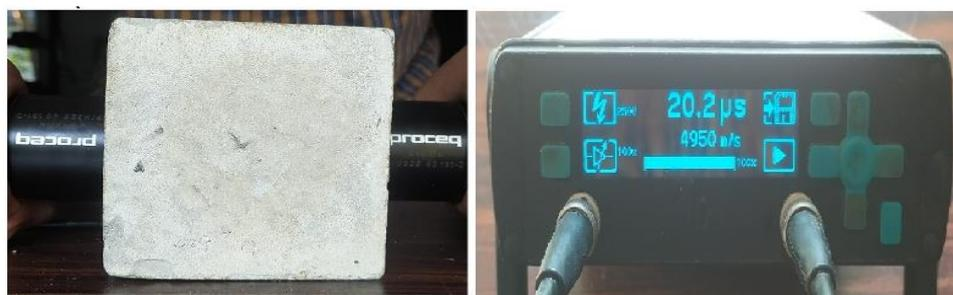
**Figure 4.** UPV test equipment used in the study.
