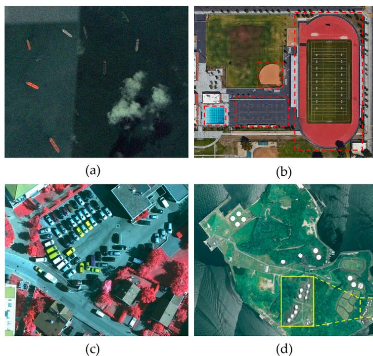
**Figure 1.** Several challenging examples. (a) The image contains noise, clouds, and light and shadow effects. (b) There is a significant variation in the scale of the objects in the image. (c) The objects are distributed in arbitrary directions in the image. (d) The image contains extremely challenging small objects.
