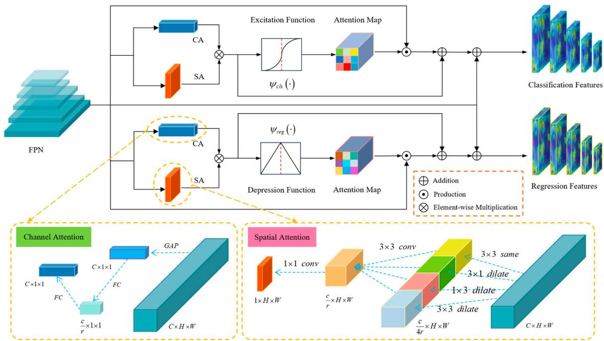
**Figure 6.** The structure and flow of the FPM. CA and SA in the figure represent channel attention and spatial attention, respectively.
