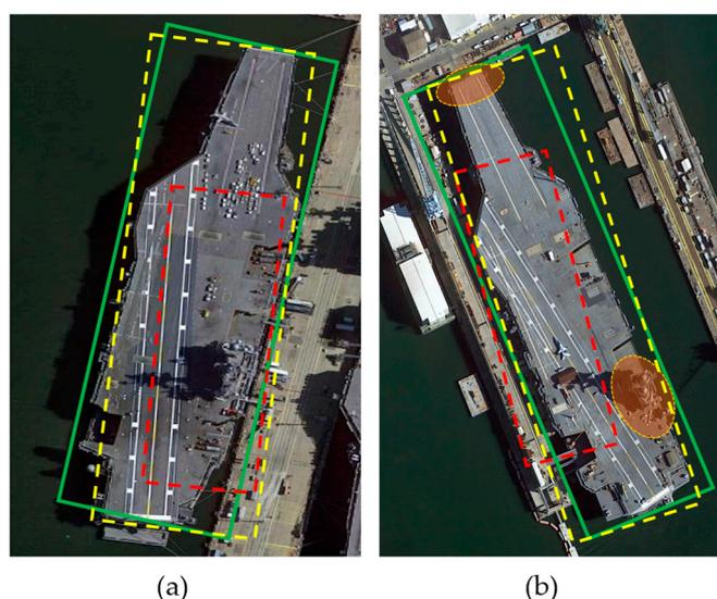
**Figure 2.** In both (a,b), the green boxes represent the ground truth boxes, the red boxes correspond to the prior anchors, and the yellow boxes depict the predicted boxes obtained through regression based on the prior anchors. It is evident from the figures that the object positions in both (a,b) are accurately located. Nevertheless, the classification error in (b) arises due to the prior anchor's inability to capture crucial features, such as the island and bow of the ship.
