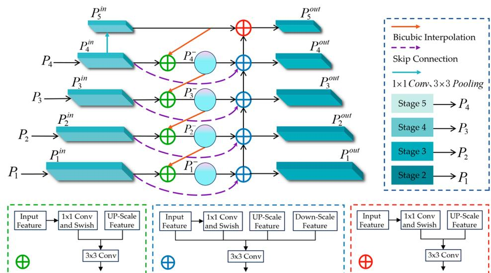
**Figure 5.** Structure and process of BMSFPN.
