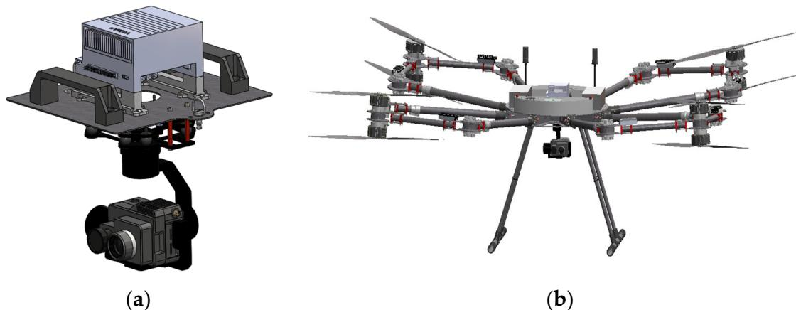
**Figure 17.** FLIR Duo PRO R: (a) dedicated custom payload case; (b) co-axial quadcopter configuration with the payload attached.
