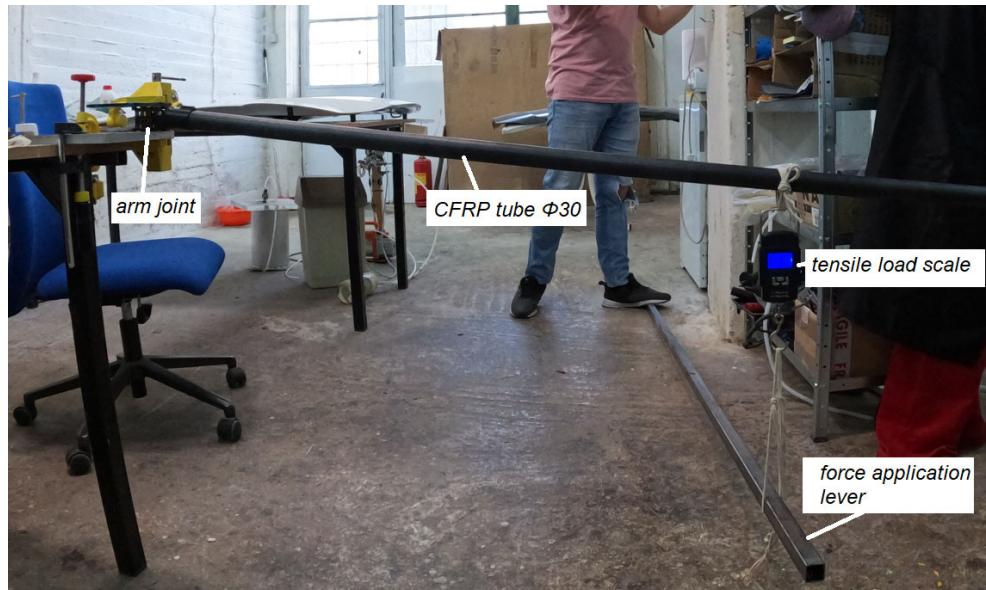
**Figure 23.** Physical testing of the aluminum joint.
