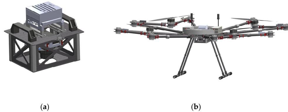
**Figure 16.** Sony A6100: (a) dedicated custom payload case; (b) quadcopter configuration with the payload attached.
