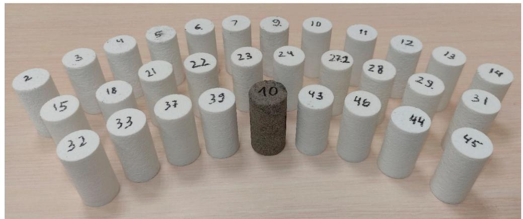
**Figure 2.** External appearance of the core (sandstone No.10) and synthetic specimens.
