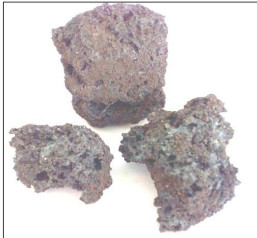
**Figure 4.** Nickel-containing composite material using nickel ore and coke.
