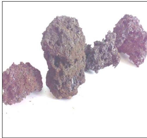
**Figure 3.** Nickel-containing composite material using nickel ore and semi-coke.
