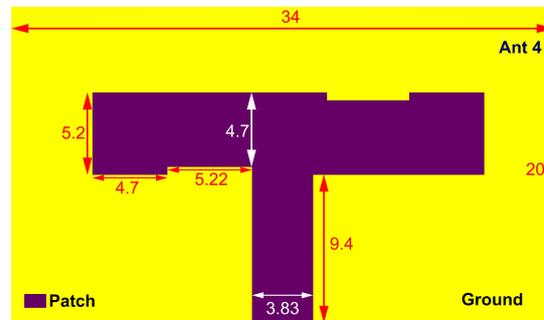
Figure 1. Dimensions of 5G FR2 (all in mm).
