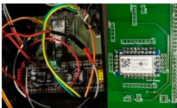
**Figure 4.** Electrochemical module prototype using PSOC 5 and ADuCM355.
