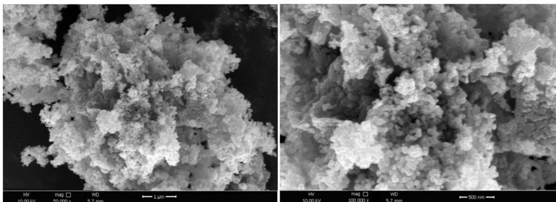
**Figure 4.** SEM images of resulting  $\text{CuCo}_2\text{S}_4/\text{CuCo}_2\text{O}_4$  heterostructure.
