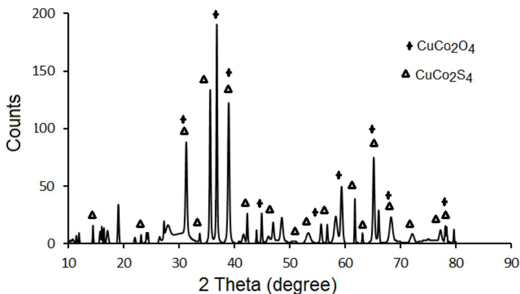
**Figure 2.** XRD pattern of the prepared  $\text{CuCo}_2\text{S}_4/\text{CuCo}_2\text{O}_4$  nanoparticles.
