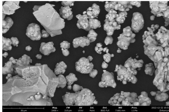
**Figure 2.** Grit blasting after 20× magnification.
