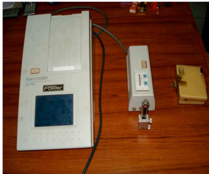
**Figure 3.** SurfCorder SE 1700 (surface roughness measuring instrument), Automation and Metrology Inc., Mentor, OH, USA.
