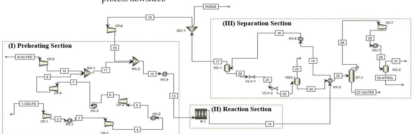
**Figure 1.** Process flowsheet of CO<sub>2</sub> hydrogenation to methanol [13].
