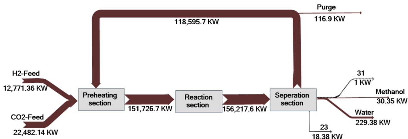
Figure 2. Grassmann diagram of all three sections of CTM plant.
