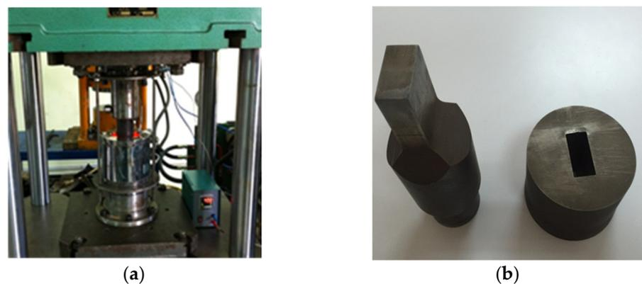
**Figure 3.** Scheme of the CCDF set-up and tools: (a) experiment die; (b) punch and die.
