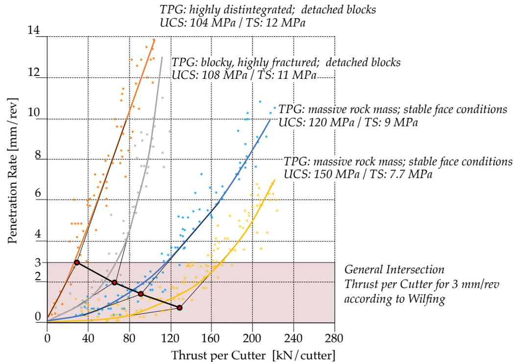
**Figure 1.** Compilation of the penetration tests carried out on the Koralm Basetunnel for various UCS values and fracturing classes (modified after Wilfing (2016)) [12].
