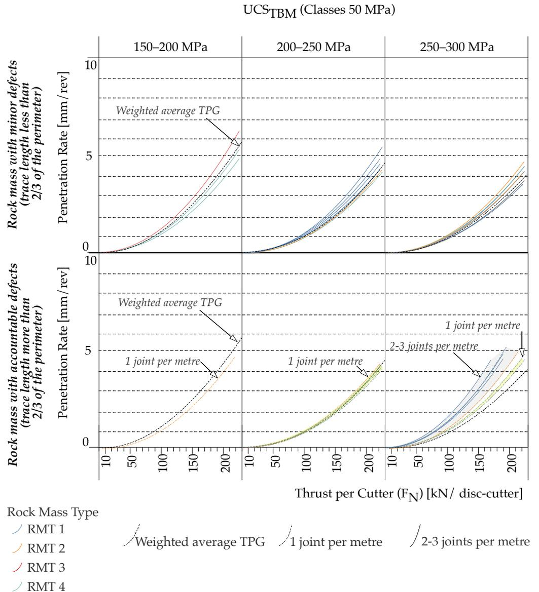
**Figure 5.** Correlation between Uniaxial Compressive Strength (UCS) and rock mass conditions, categorized into rock mass with minor defects (trace lengths less than 2/3 of the perimeter) and rock mass with significant defects (trace lengths more than 2/3 of the perimeter). The selection of UCS tests for TBM Penetration Rate analyses is based on the methodology of Wannemacher et al. [26].
