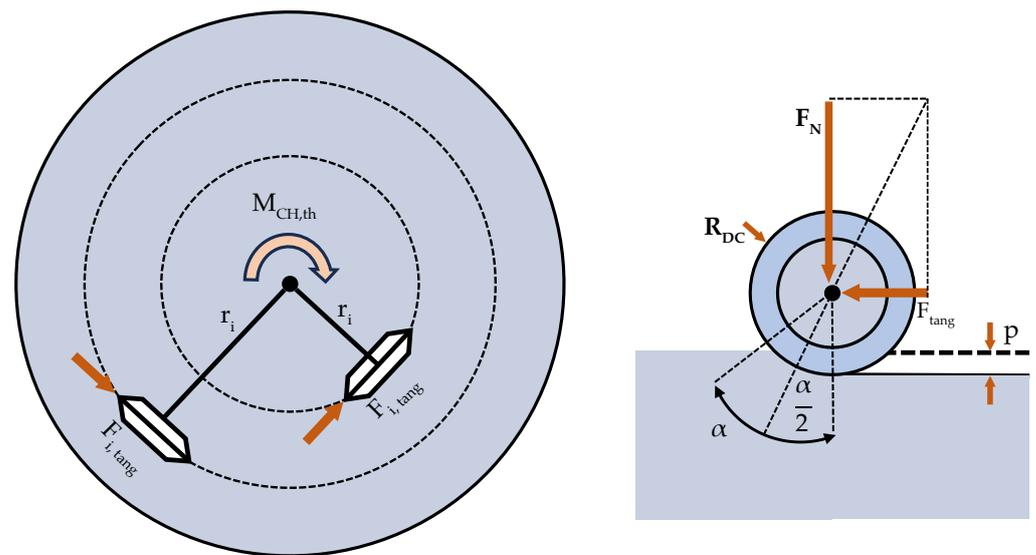
**Figure 3.** Left: Theoretical cutterhead torque  $M_{CH,th}$ . Right: Relationship between  $F_{normal}$ ,  $d_{penetration}$ ,  $r_{cutter}$ , and  $F_{tangential}$  (modified after Radončić et al. [7] and Heikal et al. [20]).
