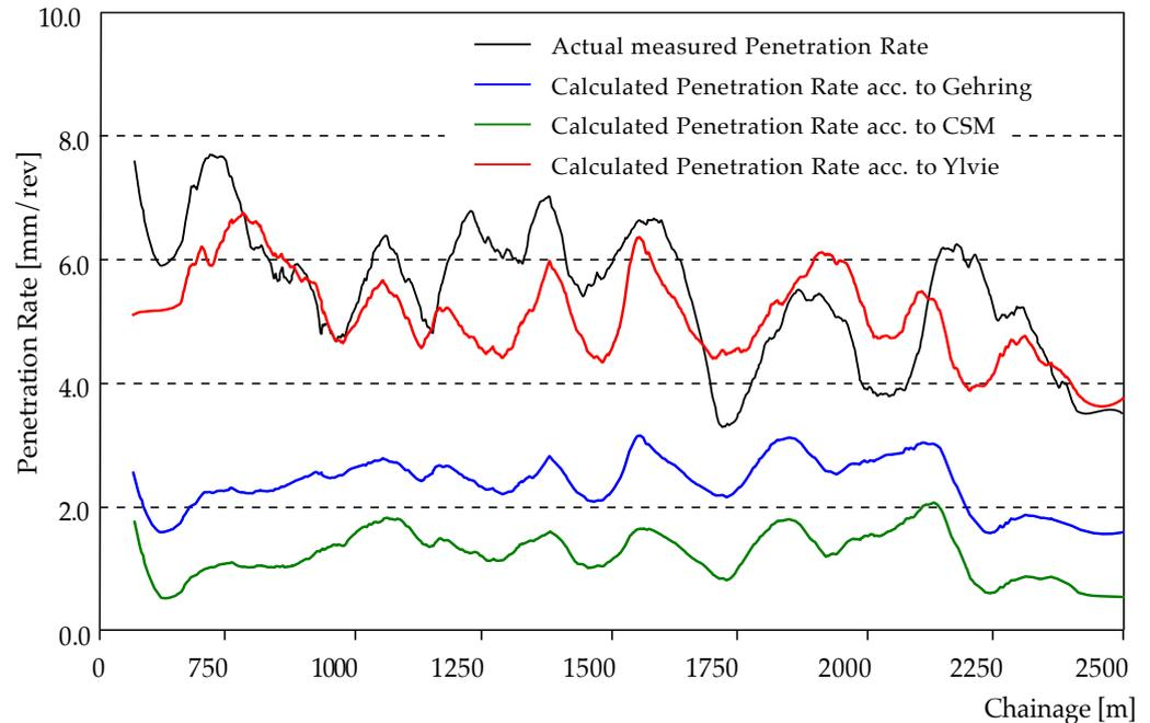
**Figure 7.** Comparison of penetration rate values calculated using the CSM model, Gehring model, and the matrix approach introduced in this paper, which is based on the Ylvie model, with the actual penetration measurements. The penetration rate consistently corresponds to the Thrust per Cutter as detailed in Figure 6 [21].
