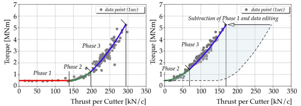
Figure 4. Exemplary stroke before (left) and after (right) reduction in friction according to the Ylvie model.
