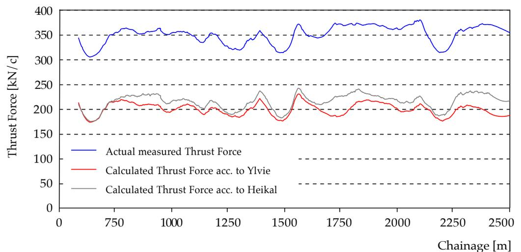
**Figure 6.** Comparison of Thrust per Cutter values calculated using the model proposed by Heikal et al. [20] and the Ylvie model approach introduced in this paper, with the actual measured values [21].
