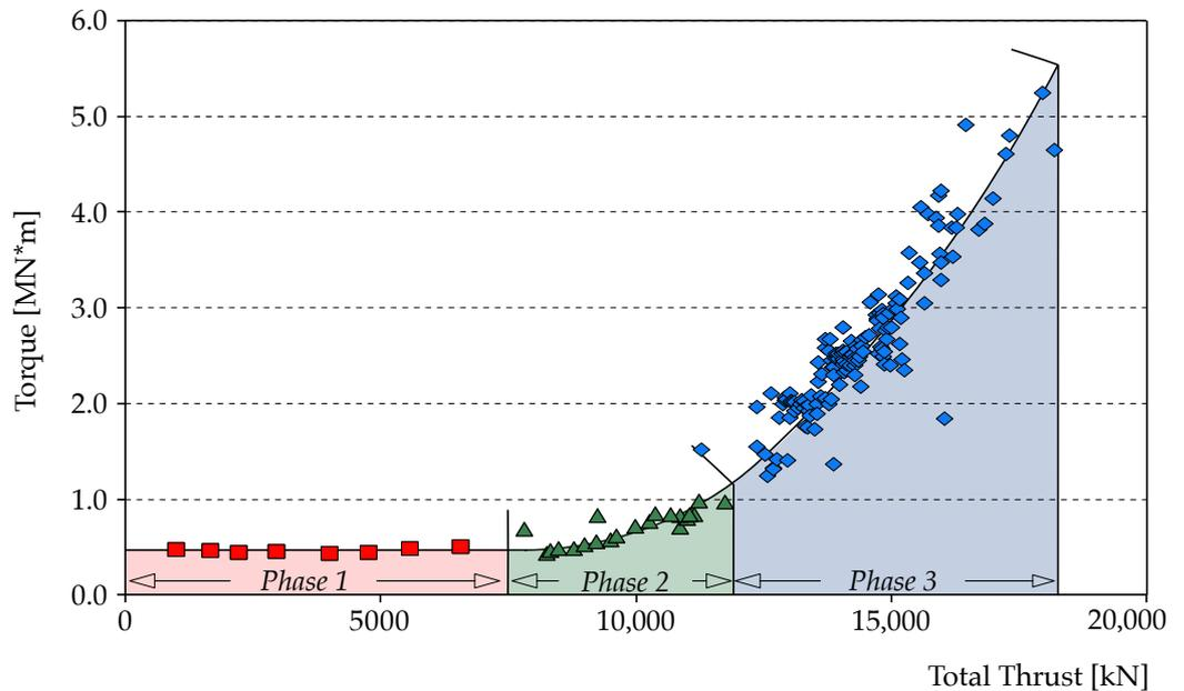
**Figure 2.** Determination of the friction force according to Wild [13].
