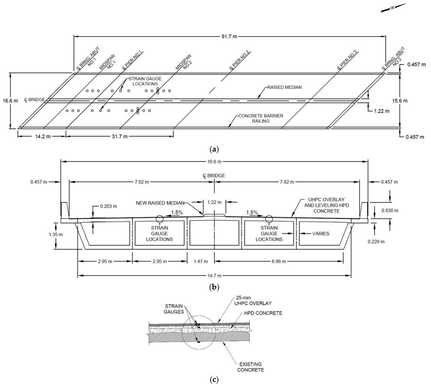
**Figure 4.** Bridge design layout with sensor instrumentation—(a) plan view; (b) cross-sectional view and (c) deck cross-sectional view.
