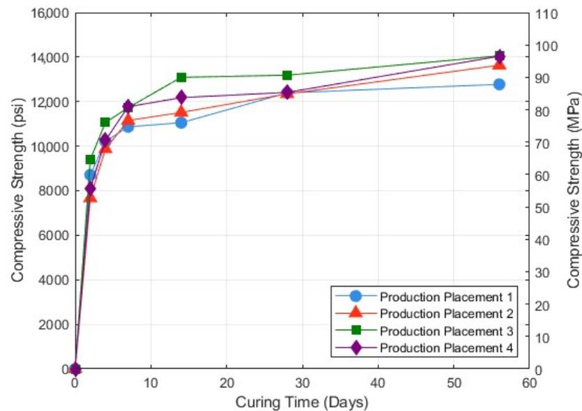
Figure 12. All production placements—compressive strength gain.
