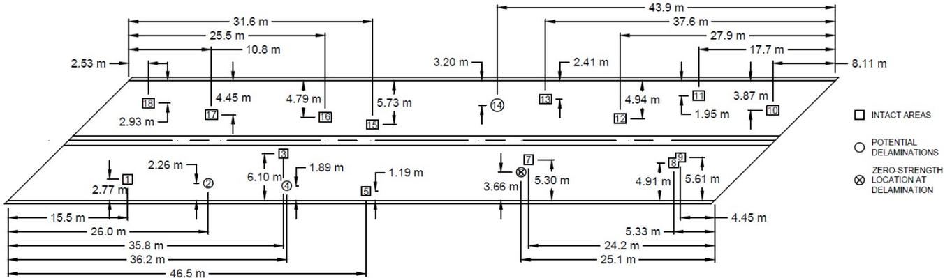
Figure 15. Direct tension pull-off tests conducted on bridge no. 7032.
