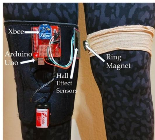
**Figure 8.** Prototype of a wearable Hall sensor for gait monitoring. Reprinted from [102], originally published under a CC-BY license.
