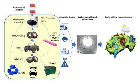
**Figure 4.** LCA framework for car tire production and microplastic release in real-world scenarios. The yellow box represents the stage where MPs are actively produced and subsequently released through major pathways.
