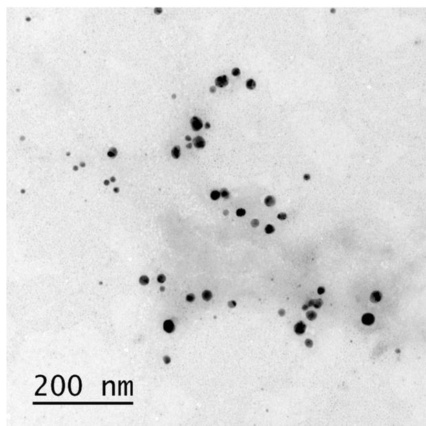
**Figure 1.** Characterization using transmission electron microscopy (TEM) of bio-AgNP suspensions synthesized with *F. oxysporum* and deposited in a copper sample port coated with parlodium film at 200 nm.
