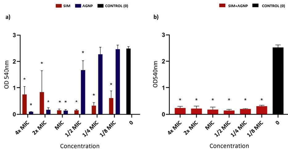
**Figure 2.** Graph (a) represents biofilm inhibition for SIM and bio-AgNP and graph (b) represents biofilm inhibition by association at concentrations from 4× to 1/8 MIC for the standard *S. aureus* ATCC 29213 strain after 24 h. The expressed values refer to the mean and standard deviation of the absorbance readings (OD 540 nm). \* indicates statistical differences from the control. (ANOVA, 2 criteria, Tukey). Column “0” indicates the growth of the untreated standard ATCC 29213 strain.
