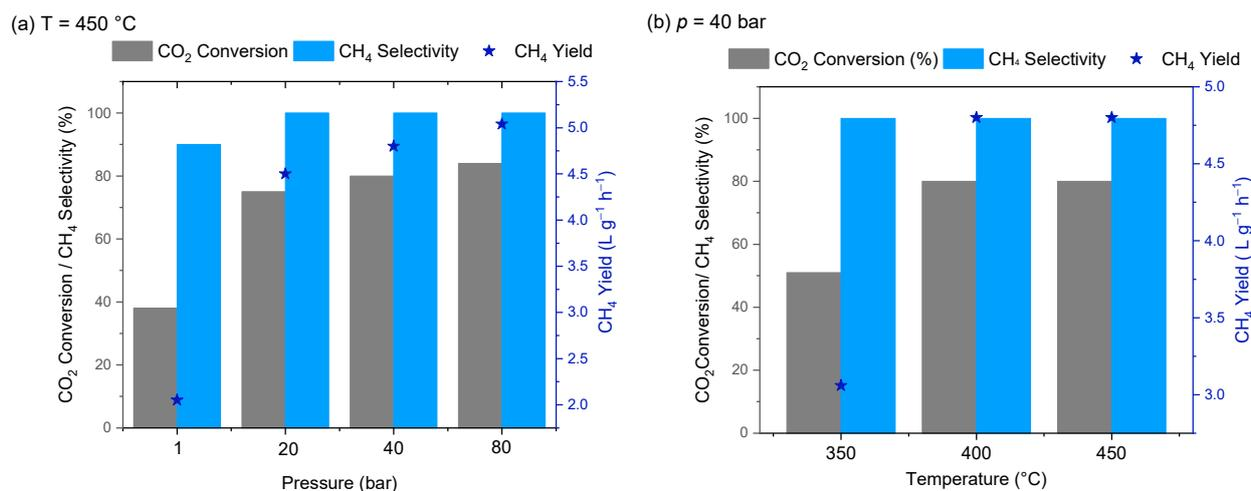
**Figure 4.** (a) Effect of pressure at 450 °C and (b) effect of temperature at 40 bar on CO<sub>2</sub> methanation over Ni/Al<sub>2</sub>O<sub>3</sub>-HTC. Reaction conditions: fixed-bed reactor packed 200 mg of Ni/Al<sub>2</sub>O<sub>3</sub> pre-reduced at 500 °C, CO<sub>2</sub>:H<sub>2</sub> = 1:4, GHSV = 30,000 mL·g<sub>cat</sub><sup>-1</sup>·h<sup>-1</sup>.
