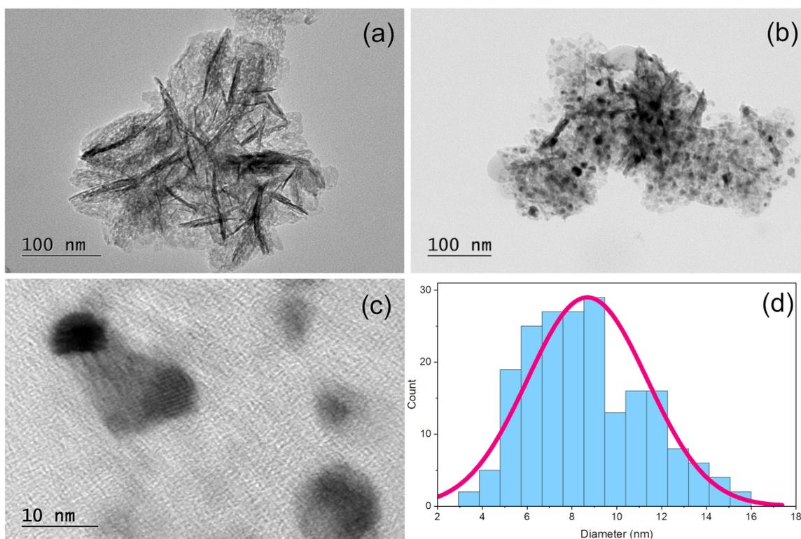
**Figure 2.** Transmission electronic microscopy (TEM) images of Ni/Al<sub>2</sub>O<sub>3</sub>-HTC (a) as-prepared; (b,c) reduced at 500 °C under H<sub>2</sub>; (d) histogram size distribution of Ni nanoparticles.
