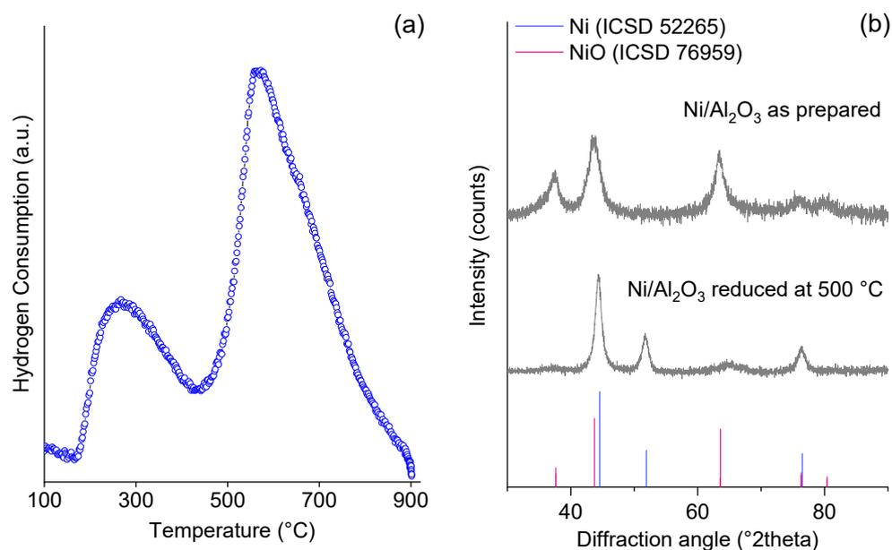
**Figure 1.** (a) Temperature-programmed reduction (TPR) of as-prepared Ni/Al<sub>2</sub>O<sub>3</sub>-HTC; (b) XRD pattern of the Ni/Al<sub>2</sub>O<sub>3</sub> catalyst as prepared and reduced at 500 °C.
