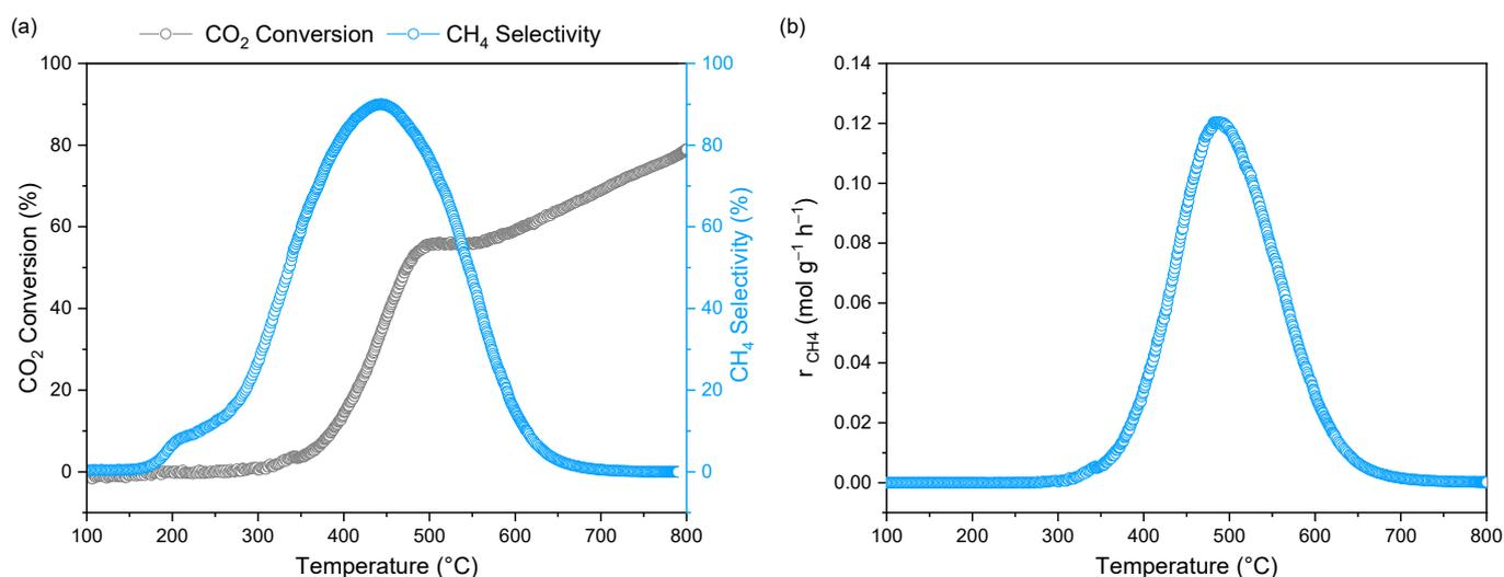
**Figure 3.** Effect of temperature on CO<sub>2</sub> hydrogenation at atmospheric pressure over Ni/Al<sub>2</sub>O<sub>3</sub>-HTC. Reaction conditions: Ni/Al<sub>2</sub>O<sub>3</sub>-HTC pre-reduced at 500 °C, atmospheric pressure, CO<sub>2</sub>:H<sub>2</sub> = 1:4, GHSV = 30,000 mL·g<sub>cat</sub><sup>-1</sup>·h<sup>-1</sup>. (a) CO<sub>2</sub> conversion and CH<sub>4</sub> selectivity; (b) CH<sub>4</sub> production rate.
