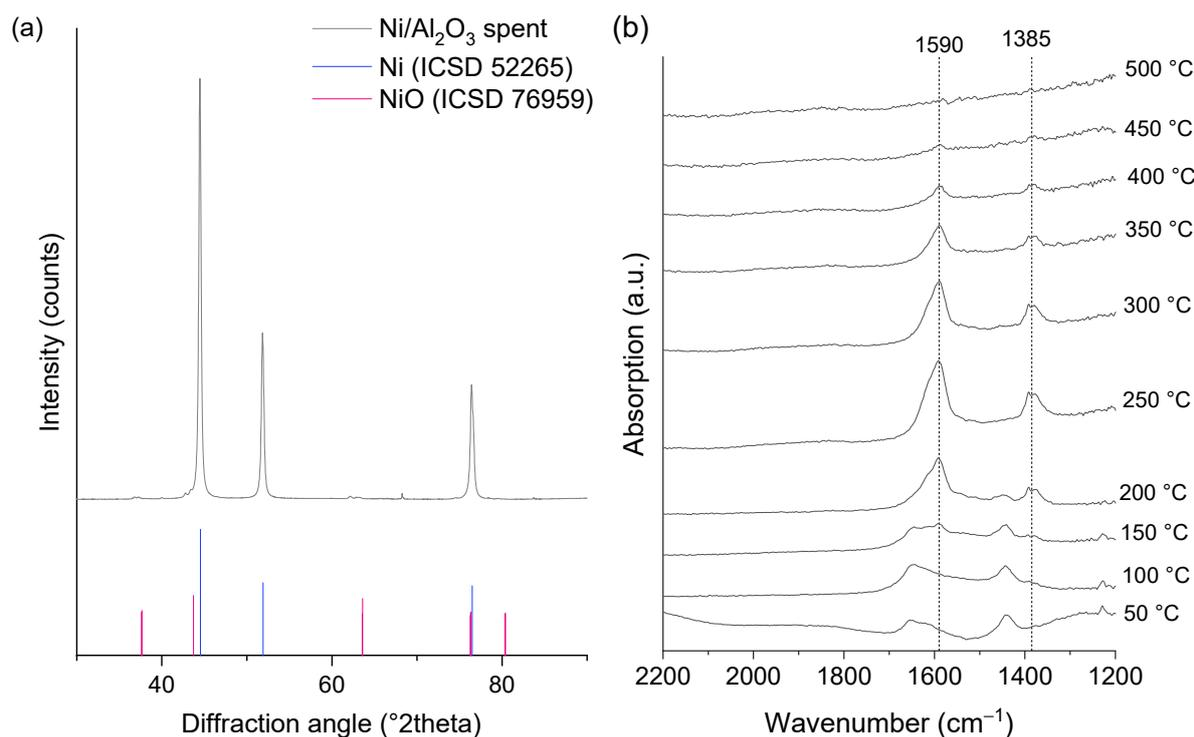
**Figure 6.** (a) XRD pattern of the Ni/Al<sub>2</sub>O<sub>3</sub>-HTC catalyst spent after CO<sub>2</sub> hydrogenation to CH<sub>4</sub> at 400 °C and 40 bar; (b) DRIFTS of CO<sub>2</sub> methanation reaction over Ni/Al<sub>2</sub>O<sub>3</sub>-HTC pre-reduced at 500 °C at different temperatures, atmospheric pressure, and CO<sub>2</sub>:H<sub>2</sub> = 1:4. All spectra were baseline-corrected with spectra recorder under Ar at the same temperature.
