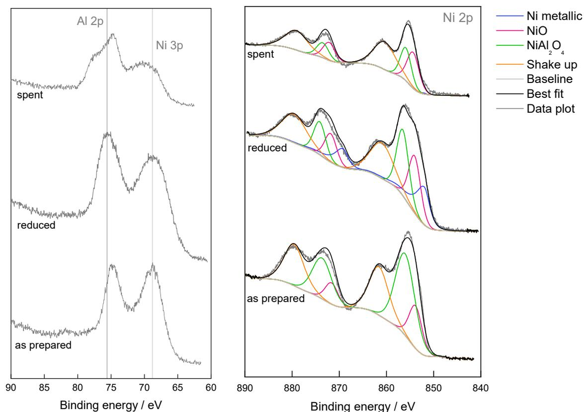
**Figure 5.** Al 2p and Ni 2p XPS of Ni/Al<sub>2</sub>O<sub>3</sub>-HTC catalyst as prepared, reduced, and spent after CO<sub>2</sub> hydrogenation at 400 °C and 40 bar. 30 scans collected at E<sub>pass</sub> = 20 eV and 0.05 eV step.
