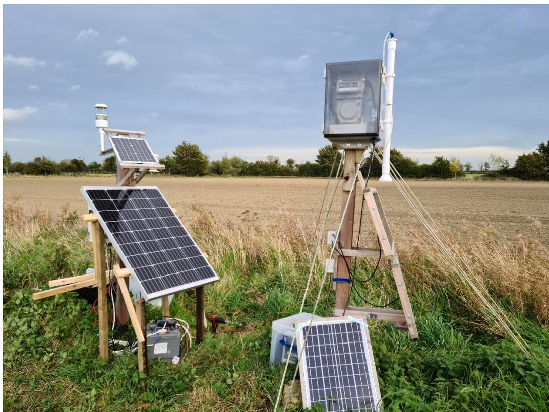
**Figure 1.** Site set-up showing DELTA II denuder system and MetOne weather station, connected to a self-sustaining power system.
