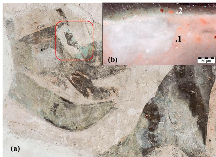
**Figure 7.** (a) Detail of St. Nicholas scene, north wall of the nave with two different green tones. Red rectangle marks a turquoise one. (b) Microphotograph of a sample cross section from the darker green area: lime-aggregate plaster (1), green colour layer with some red particles applied a fresco (2).
