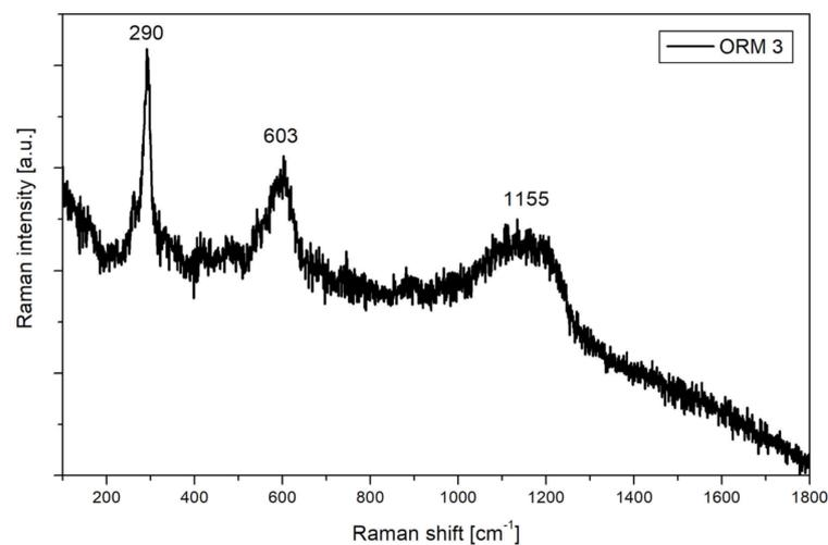
**Figure 10.** Raman spectrum of the sample ORM 3 identifying tenorite by its characteristic Raman vibrations at  $300$  and  $600\text{ cm}^{-1}$ . Sample from the first female saint's coat, lower pictorial band, triumphal wall of the nave, St. Jacob's church, Ormož, Slovenia.
