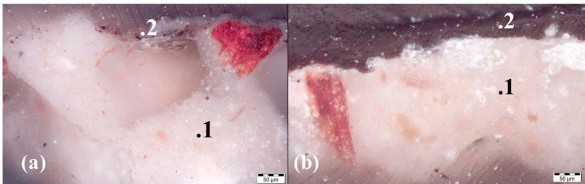
**Figure 3.** Microphotographs of sample cross sections: (a) ORM 9: plaster of lime and aggregate (1), grey-pink colour layer (2), bordure between the upper and lower pictorial band; (b) ORM 4: plaster of lime and aggregate (1), thick brown colour layer, copper pigment degradation (2), column between the first two female saints on the lower pictorial band. Triumphal wall of the nave, St. Jacob's church, Ormož, Slovenia.
