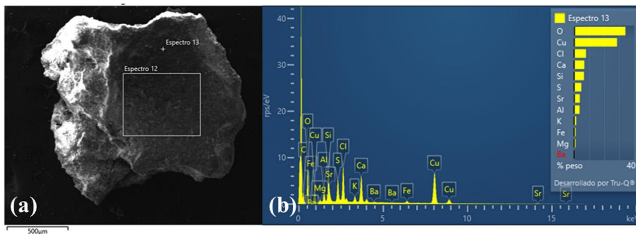
**Figure 8.** Raw sample ORM 11. (a) SEM image with marked point (13) and area (12) of EDS analysis; (b) EDS spectrum of the point analysis indicating the presence of green earth (Mg, Al, Si, S, K, Fe) and malachite (Cu) degraded to (para)atacamite (Cu, Cl). Sample from the green background, north wall of the nave, St. Jacob's church, Ormož, Slovenia.
