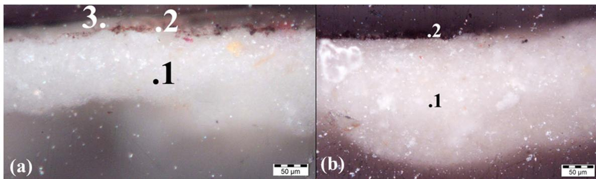
**Figure 11.** Microphotographs of sample cross sections: (a) ORM 12: lime from the plaster (1), red-brownish (probably degraded pigment) colour layer a fresco (2), white colour layer a fresco (3), St. Martin scene, north wall. (b) ORM 10: lime from the plaster (1), darkened colour layer (2), decoration bordure under the four female saints. Triumphal wall of the nave, St. Jacob's church, Ormož, Slovenia.
