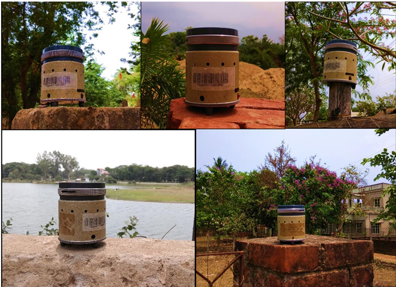
**Figure 1.** Aerobiological sampling by Burkard personal volumetric sampler at different sampling locations of Santiniketan.
